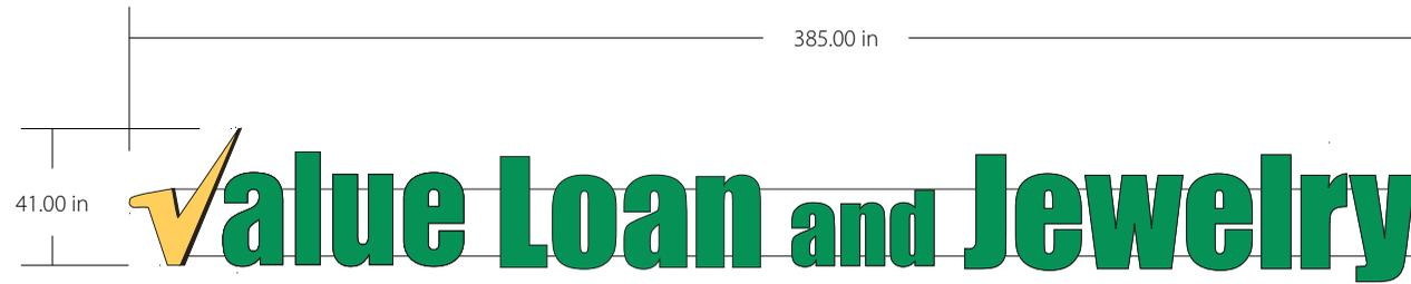
LED Illuminated Channel Letters on Raceway
